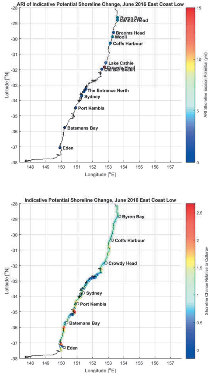
**Figure 12. (upper) Estimated ARI (years) of coastal erosion and (lower) shoreline change potential relative to Collaroy for the June 2016 East Coast Low.**
