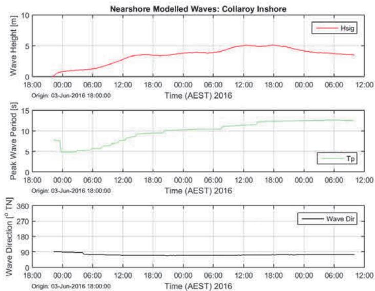
Figure 6. Nearshore modelled wave time series for Collaroy from WW3 simulation.
