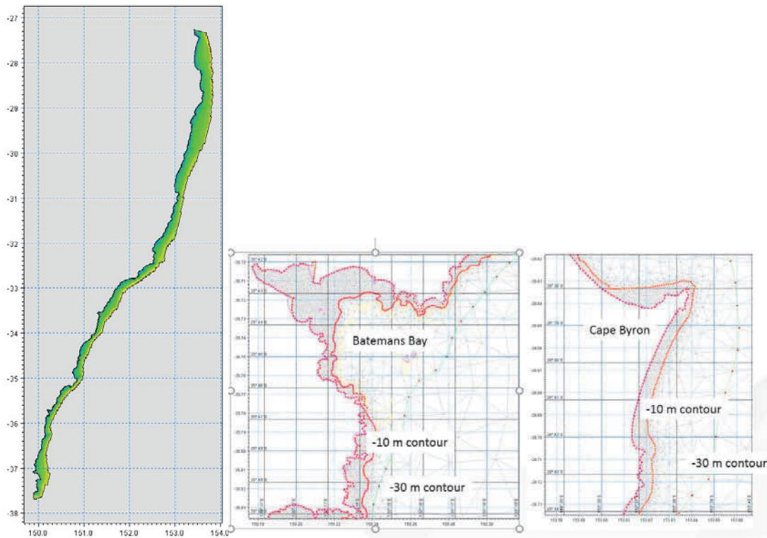
**Figure 4. (left) Extents of the NSW-wide nearshore wave unstructured mesh and (right) close-up showing resolution of elements at Batemans Bay and Byron Bay.**
