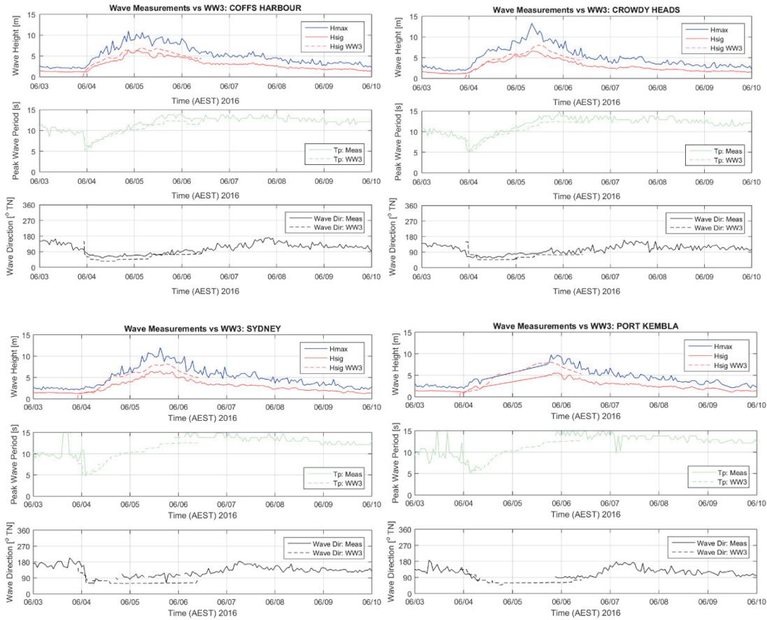
Figure 5. Modelled vs measured wave parameters at selected NSW offshore wave buoys between 4th and 9th June 2016 (measurements: MHL).
