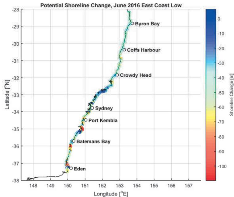
**Figure 10. Estimated shoreline change potential (m) (negative = erosion, positive = accretion) for the June 2016 East Coast Low.**
