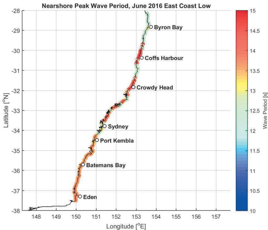
**Figure 7. Modelled nearshore peak wave parameters for the June 2016 East Coast Low: (left) Significant wave height and (right) Wave period.**
